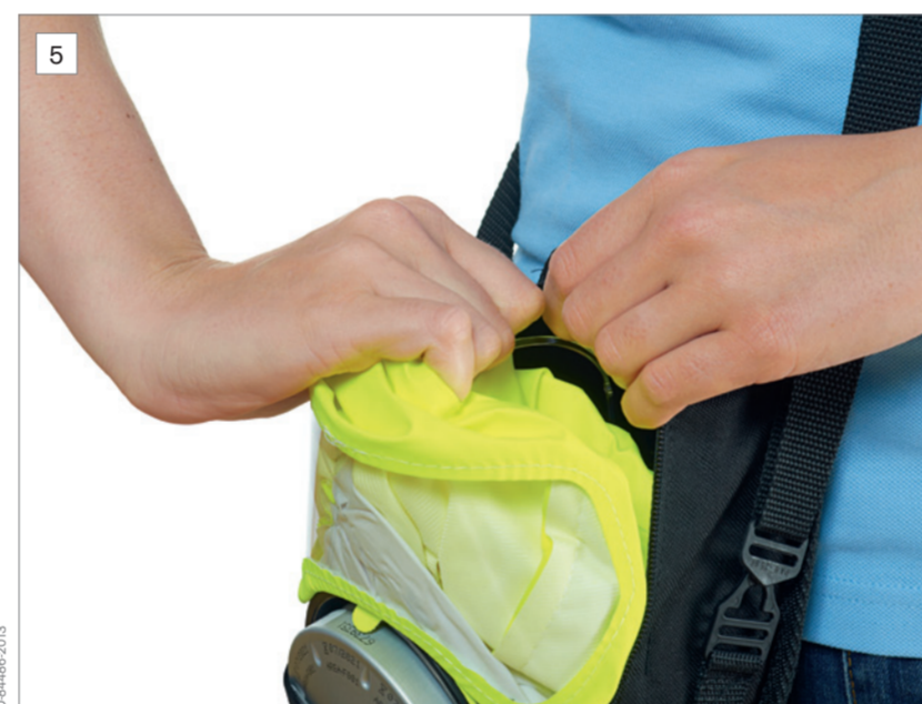
5 Remove the hood from the Soft Pack. Pull the hood against the hook and loop fastener holder, it will automatically open. The second filter sealing plug will automatically be detached when the hood is removed.
