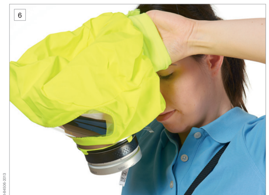
6 Widen the neck seal and pull the hood over your head. The inner head harness automatically adjusts to your head. Ensure that nose and chin sit comfortably in the half mask and that all hair is tucked into the hood.
