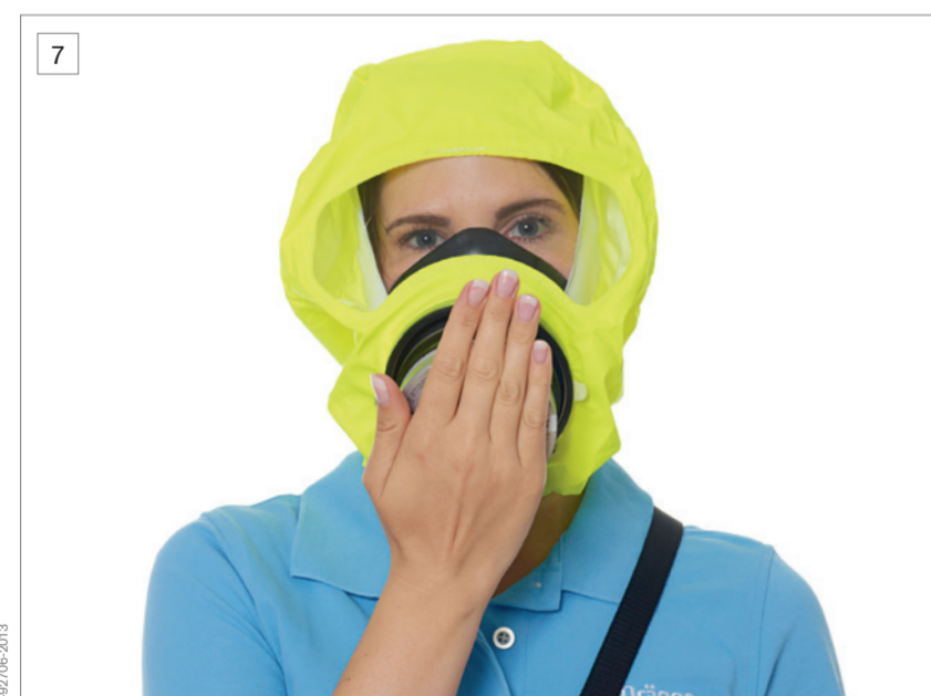
7 Check the fit of the half mask by closing the front filtering opening with the palm of your hand. If negative pressure is not generated readjust the half mask to ensure a close fit over nose and mouth.
