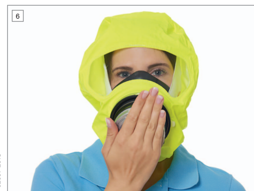
Check the fit of the half mask by closing the front filtering opening with the palm of your hand. If negative pressure is not generated readjust the half mask to ensure a close fit over nose and mouth.
